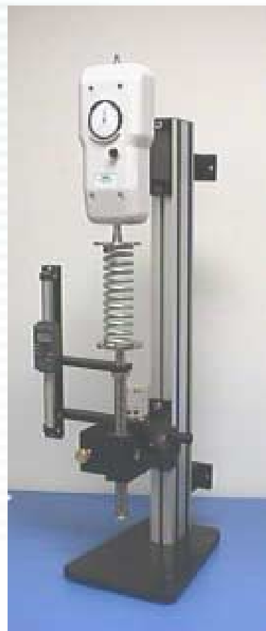
MT500H Handwheel Actuated Tester with optional Digital Indicator and Wall Mounts. Shown with DG Series force gauge.
