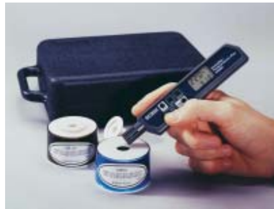
RH Pen and Calibration Standards Kit
